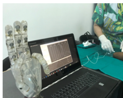
Fig. 3. Patient training for F5 finger control from a neuroprosthesis [10]
