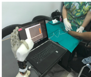
Fig. 4. Monitoring the tactile feedback signal from the fingers of neuro-prosthesis
